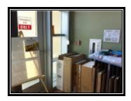
**Warehouse Area** – High level goods were found to be stored close to sprinkler heads. A minimum 18" of clearance should be maintained from stored items to ceiling mounted automatic sprinkler heads at all times.
